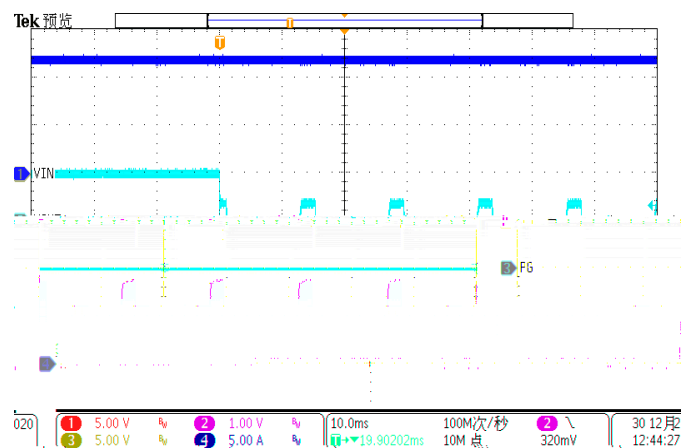
Figure 15. Over Current Protection(1A to hard short)
